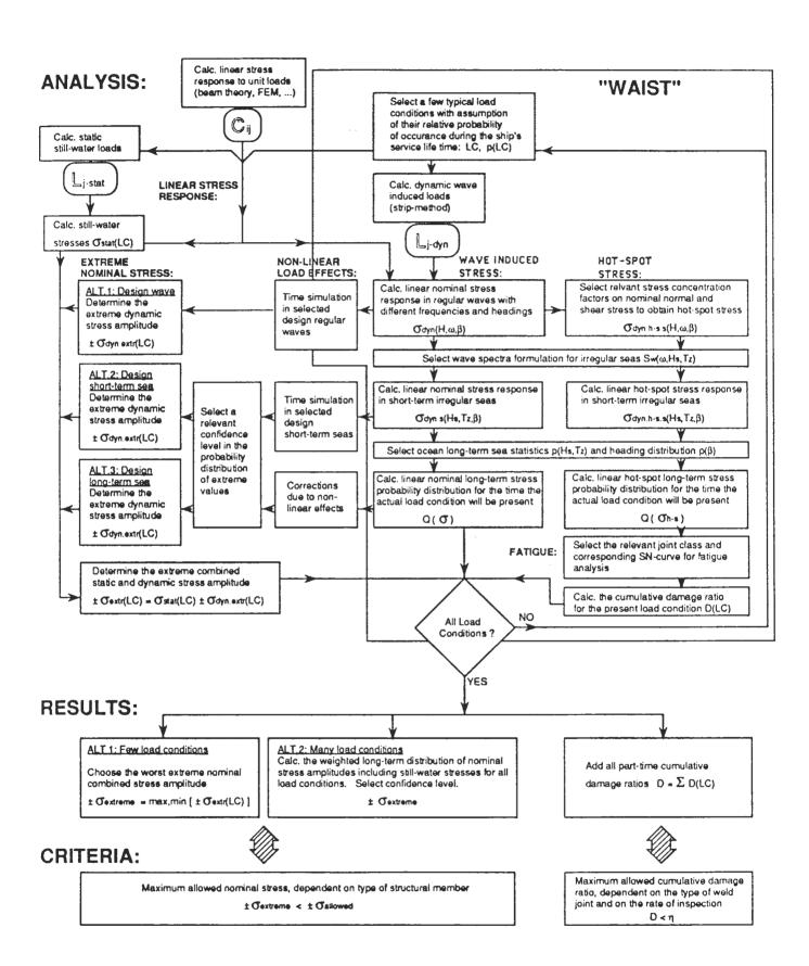
Figure 2 Flow-chart of a semi-probabilistic direct design procedure
